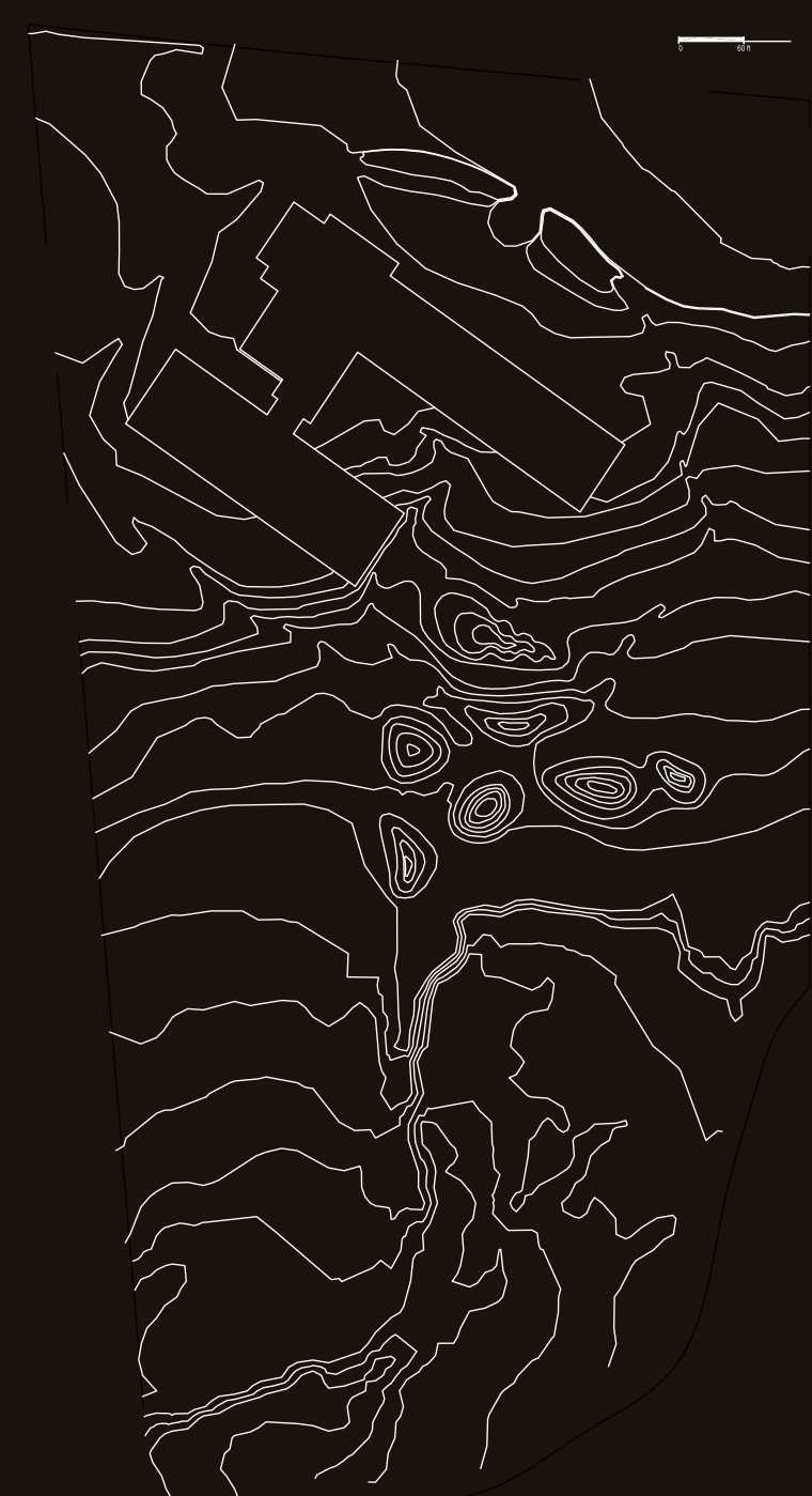
proposed topographic interventions enhance water flow through the site and provide interactive mounds from the cut and fill process of creating swales.
